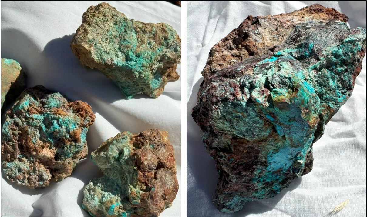
Figure 1: Odyssey rock chip samples. Sample 24PRL0123 (Left), 312 g/t Ag, 7.34% Cu, 4.34% Zn. Sample 24PRL0117 (Right), 76.1 g/t Ag, 3.48 % Cu, 24.8% Zn
