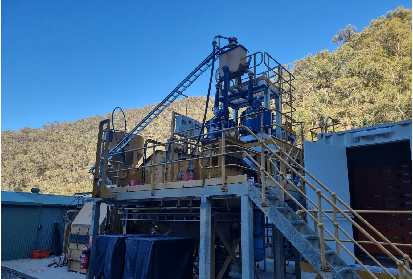
Figure 6 Side view of the gravity concentrate circuit with the gold room in the background.
