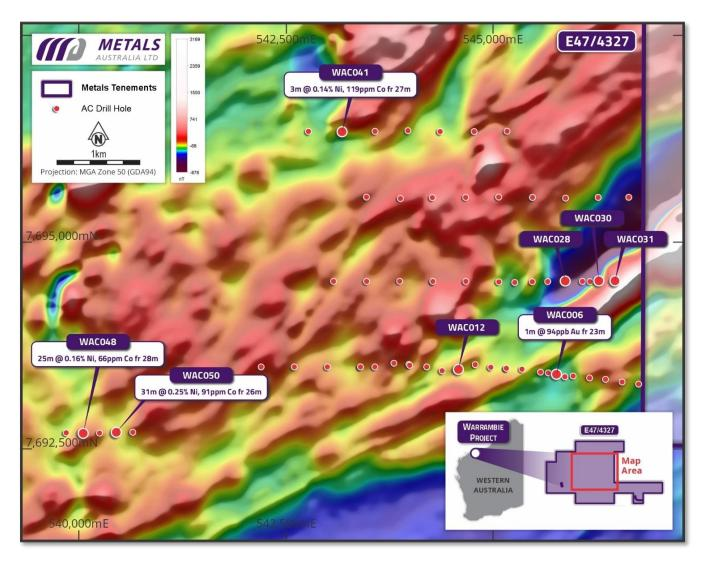
Figure 7: Warambie Project E47/4327 - reprocessed magnetics image, drill traverse targets and more significant results obtained from the phase 1 air core program completed during the 2024 campaign.
