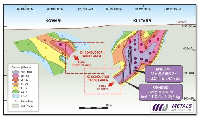
Figure 6: Long Section through the Kowari and Kultarr Zinc Ore Zones showing intercepts from holes 22MND002 and MNRC070
