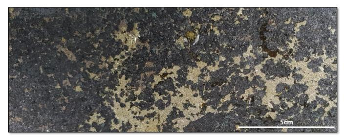
Image 1: 22MND003, 66.3m, magnetite- Ilmenite cumulate with interstitial sulphides (pyrite, pyrrhotite & chalcopyrite)
