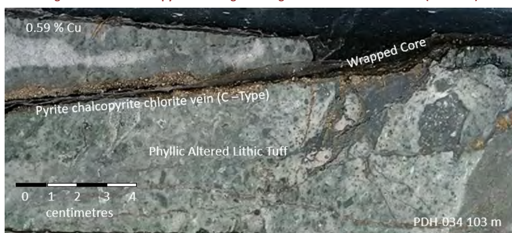
Figure 3-4. Phyllic Altered Lithic tuff with a pyrite chalcopyrite chlorite vein. (MA 2024)
