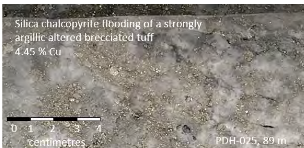
Figure 3-3. Silica chalcopyrite flooding of an argillic altered brecciated tuff. (MA 2024)
