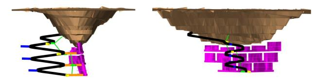
Figure 8 - Fish Underground Mine designs beneath existing open pit: Cross section looking north (left); long section looking east (right)
