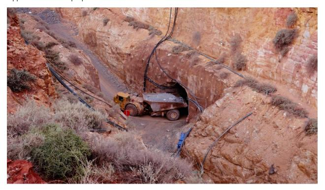
Figure 2 - Underground haul truck emerging from Second Fortune decline
