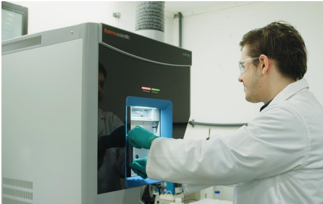
Figure 1 – ChemX's high purity Inductively Coupled Plasma Optical Emission Spectrometer (ICP-OES), under the watchful eye of ChemX Chemist Scott Stipkovich.
