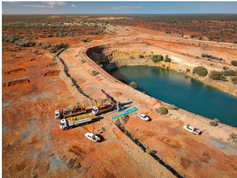
Current exploration drilling at Montague
