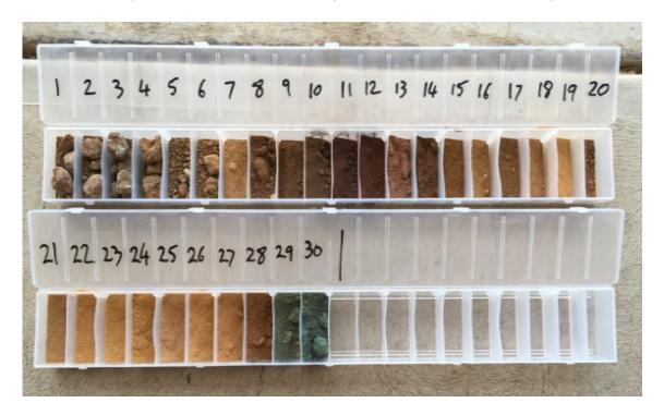
Figure 3: Chip tray for air core drill hole MA08 which intersected 9m @ 197ppm Sc from 8 metres including 3m @ 272ppm Sc from 13 metres. Numbers 1 - 30 on the chip tray denote individual downhole intervals (i.e., "10" means the drill sample obtained from 9 – 10 metres).
