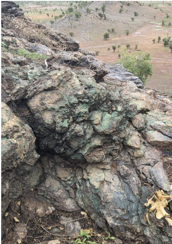
Figure 2: Left: outcropping copper mineralisation showing green copper-oxide (malachite) staining at Colline Nord, Diaguili (July 2026). Right: 100 m conductivity depth slice from the reprocessed VTEM model showing the Diaguili Conductor. Source: SGC reprocessing of 2008 Shield Mining VTEM data. Topographic contours are shown at 10m intervals.
