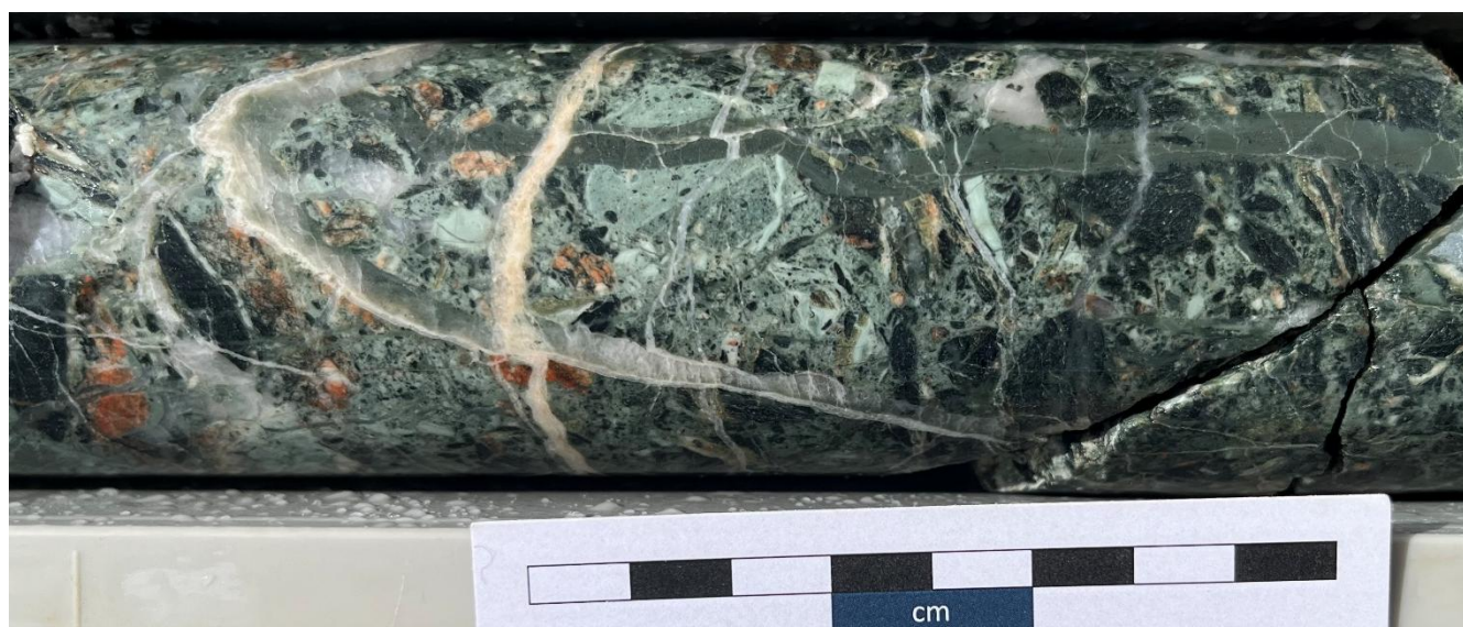
Figure 4 Portion of the Footwall Fault zone in MWD0001 (158.4-158.5m) showing multiple phases of silica-sericite alteration, brecciation and veining events. (The core in the photo has not been assayed – the same lithology intersected in RC drilling when devoid of sulphides has been unmineralised).
