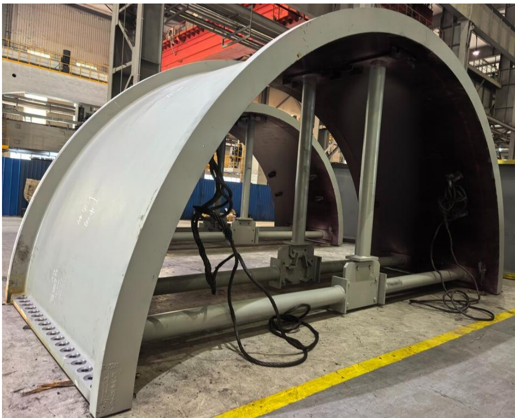
Figure 6 – SAG mill shells being fabricated
