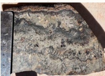
MHRK001 Colloform-crustiform quartz veining from the Mt Solitary prospect
