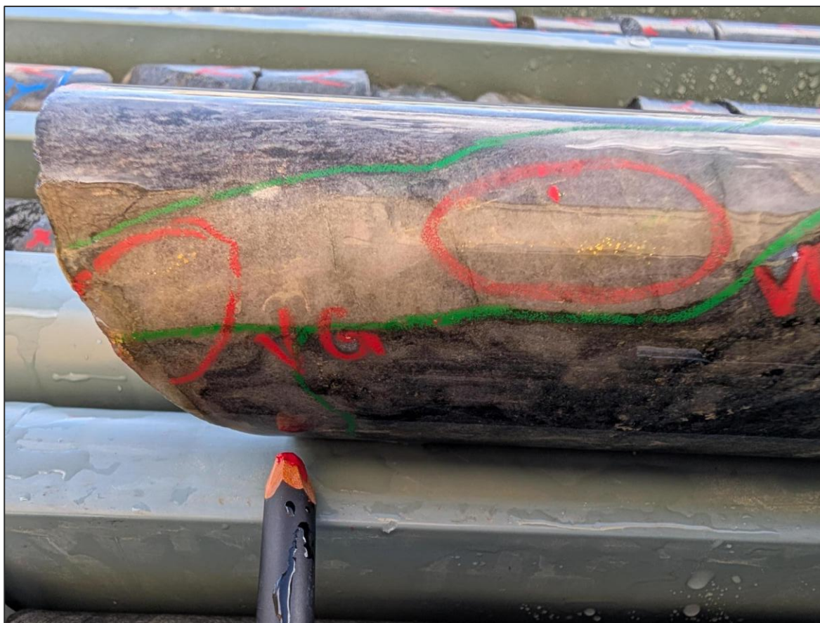
Figure 3 – Gold mineralisation located within a quartz vein hole 26HBBD044. The interval grades 4.20m @ 42.43g/t Au from 289.63m including 1.37m @ 126.93 g/t Au from 290.84m. Core width is NQ2 and ≈ 50.5mm in diameter for scale
