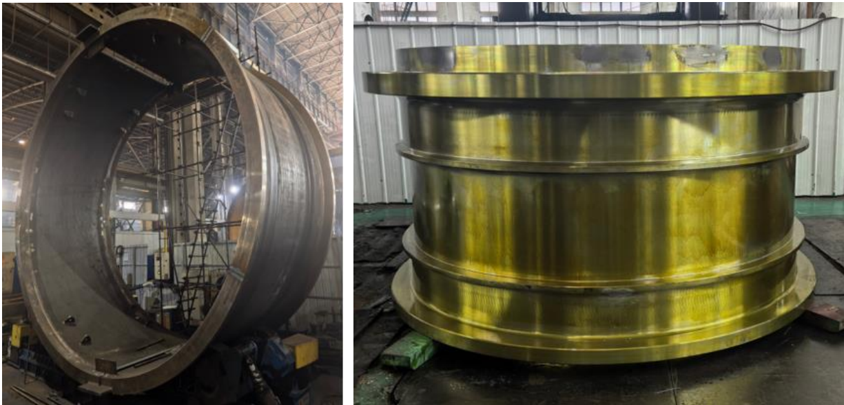
Figure 4 - Steel fabrication underway: SAG mill shell (left) and trunnion (right)
