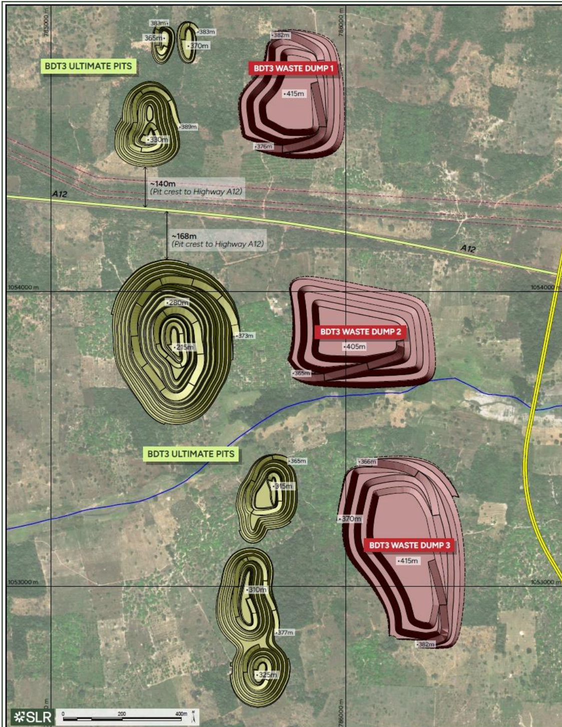
Figure 14: BDT3 Ultimate Pits and Waste Dumps
