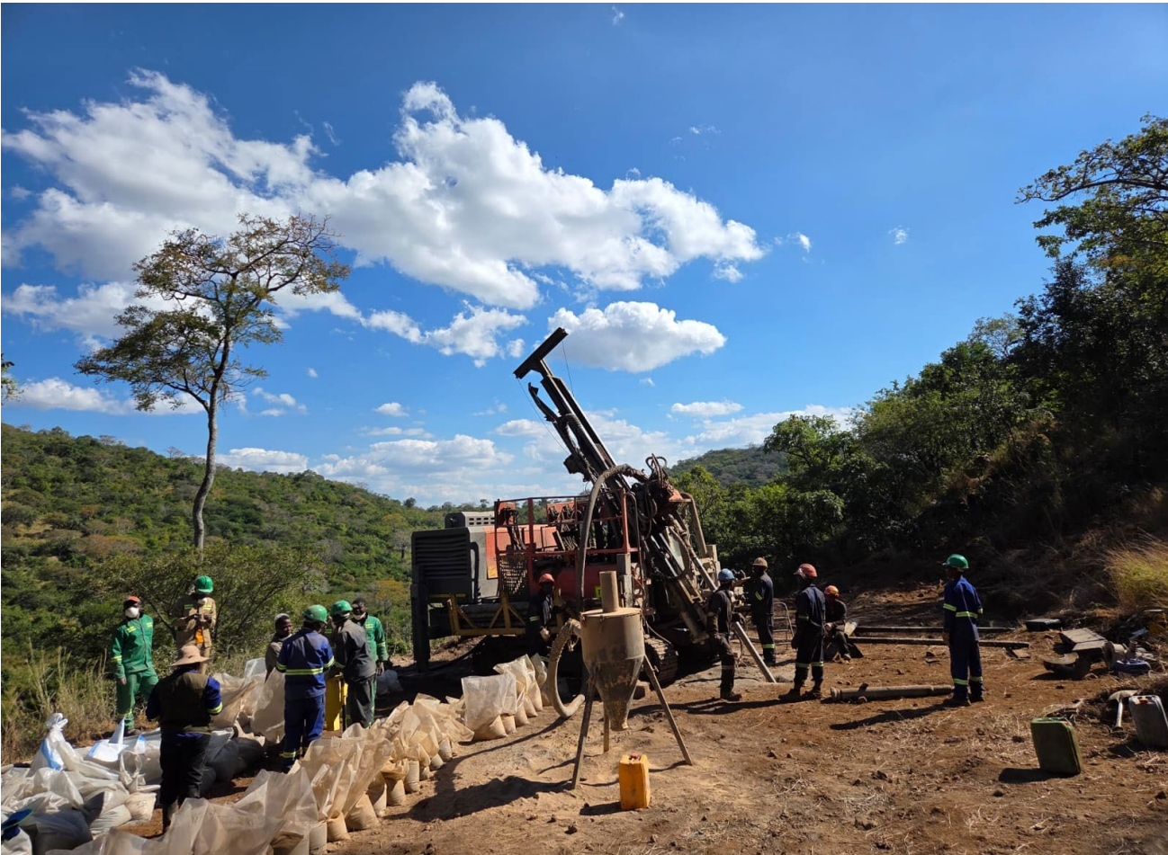
Figure 3 – Drilling continues on the second RC hole
