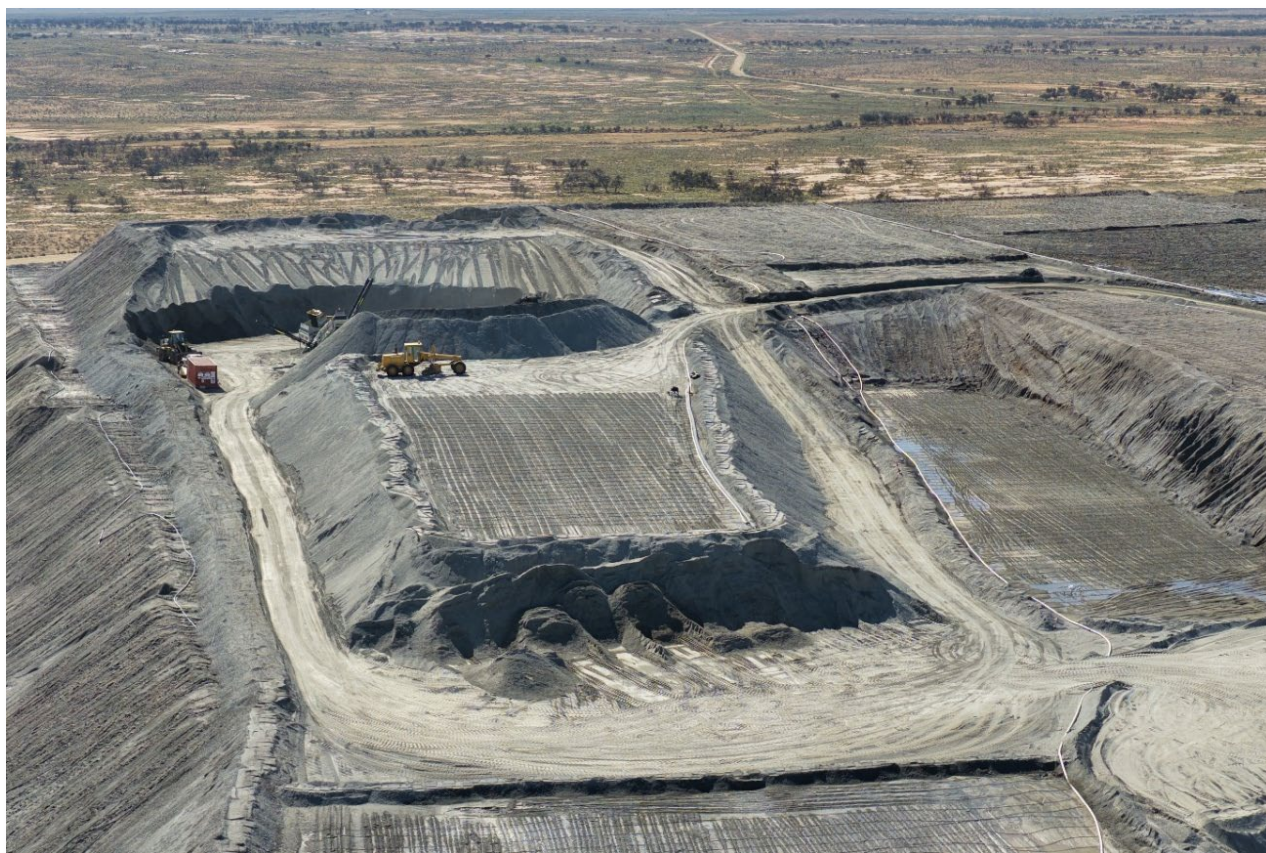
Photo 1: Photo looking north of heap leach irrigation of new re-crush material at White Dam Gold Project SA.
