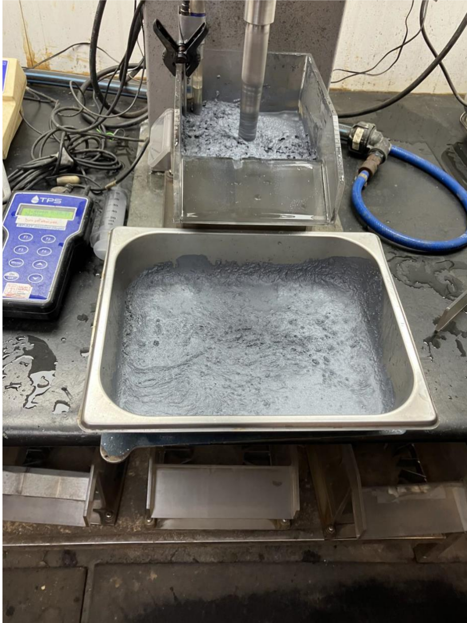
Figure 3: Composite concentrate recovered by flotation, which assayed 51.8% Sb with a 29.7% mass pull and an 85% recovery from an assayed head grade of 19.9% Sb. (Photo taken by RMX's independent consulting metallurgist Rob Riggir)
