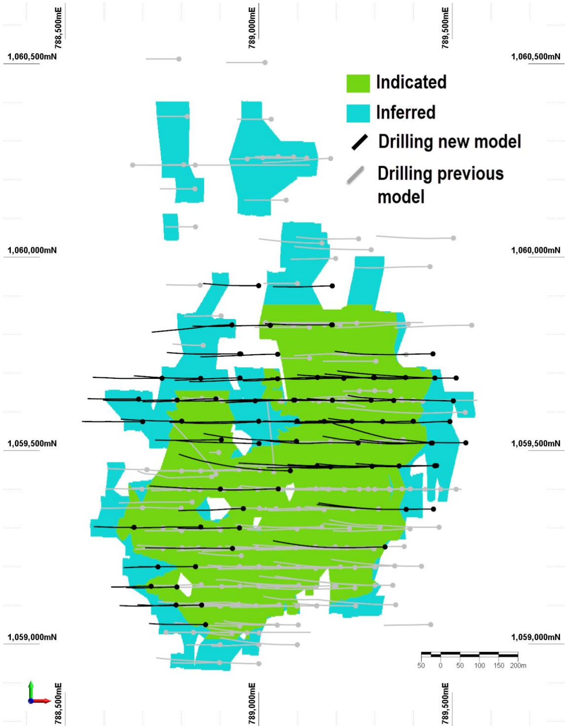
Figure 7: Plan view of BDT2 showing model classification (projected to surface with informing drilling)
