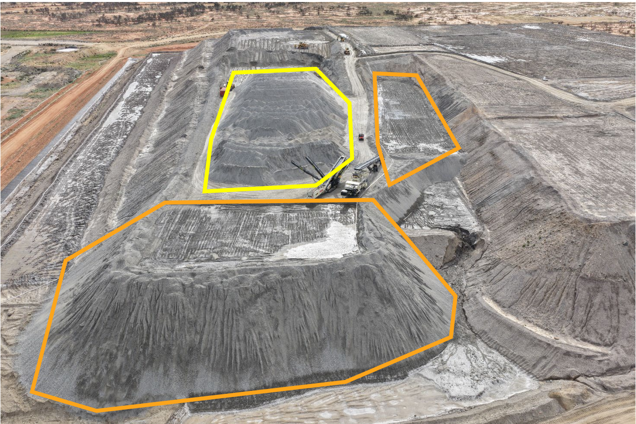
Photo 3: Newly crushed material ready for irrigation (Yellow) and newly crushed and rehandled material recently placed under irrigation (Orange) outlined on pad
