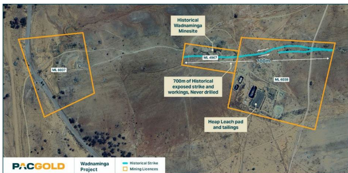
Figure 4: Wadnaminga Project area showing existing tailings and Heap Leach pads with lode location and 3 mining leases for 28.6 Ha
