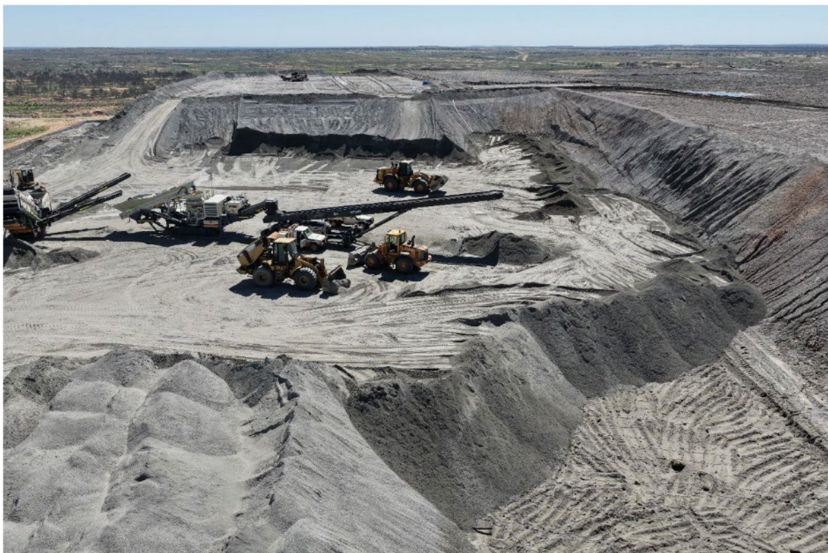
Photo 6: Re-crushing circuit in operation in south western corner of final pad lift
