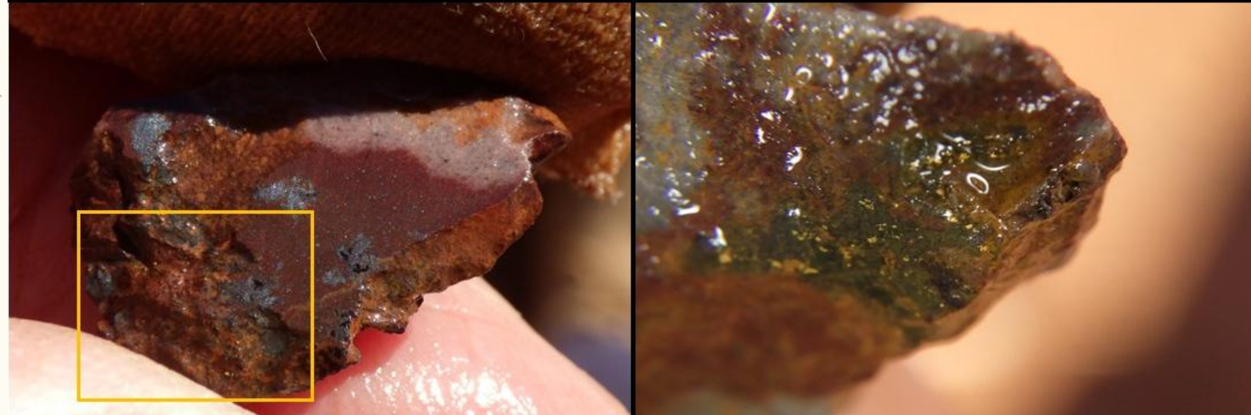
Visible gold with bismite in RC chips from Hole 25MSRC013, 46.2g/t Au from 56-57m (9)
