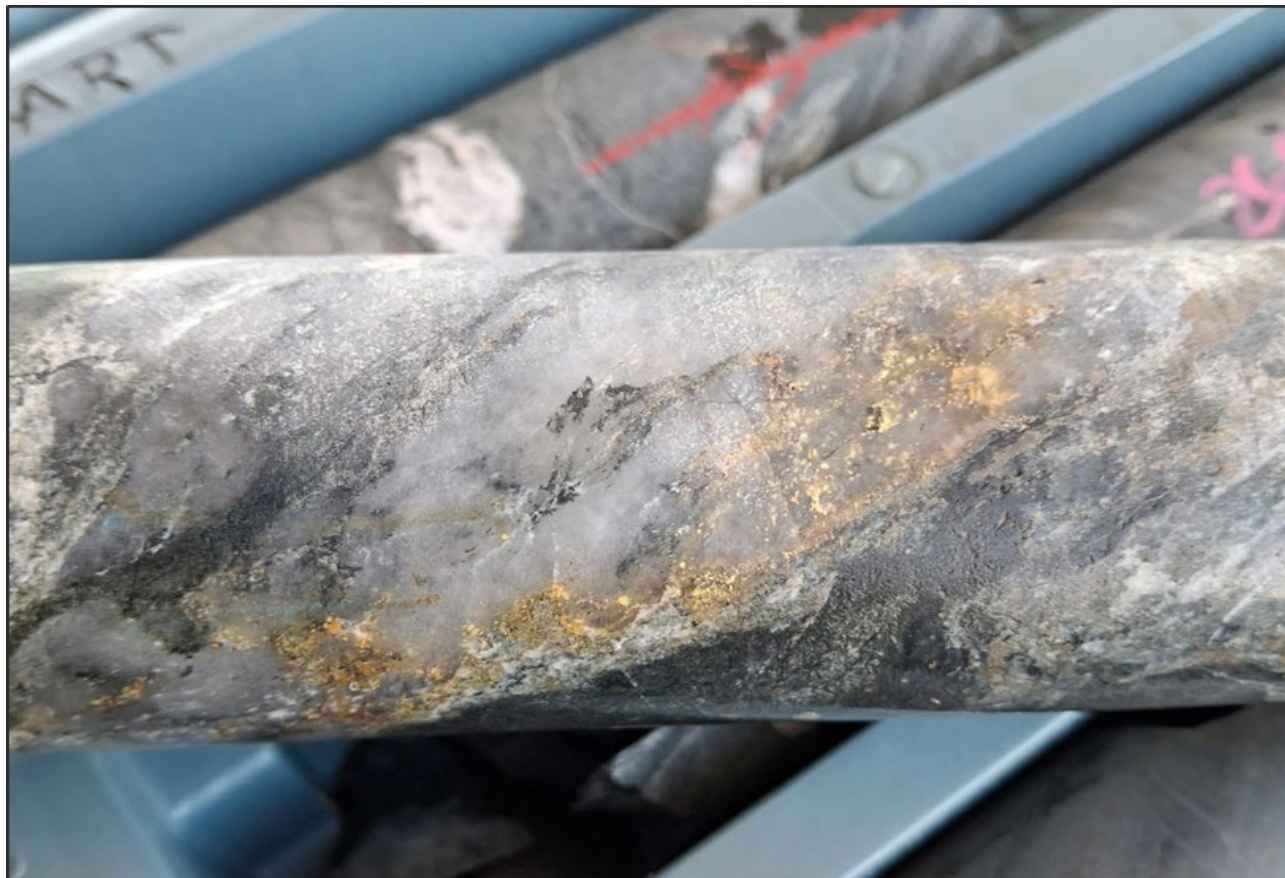
Figure 5: Visible gold in a quartz vein at 259.3m from hole 25HBBD024. The interval grades 0.3m @ 5848g/t Au from 259.17m. Core width is NQ2 and \approx 50.5 mm in diameter for scale.
