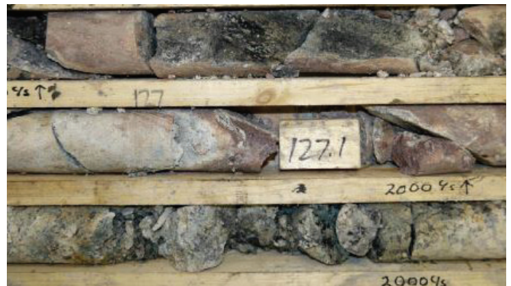
Otis West Drill Core - Similar style to Roughrider Deposit
