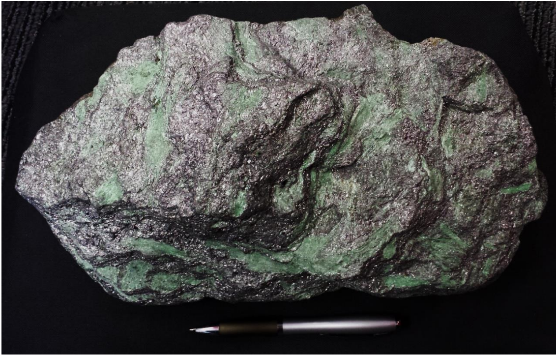
Figure 2 – Outcropping rock from the Sushi Zone containing a very high amount of green minerals. Mineralogical studies at Balama indicate that the green minerals typically host vanadium
