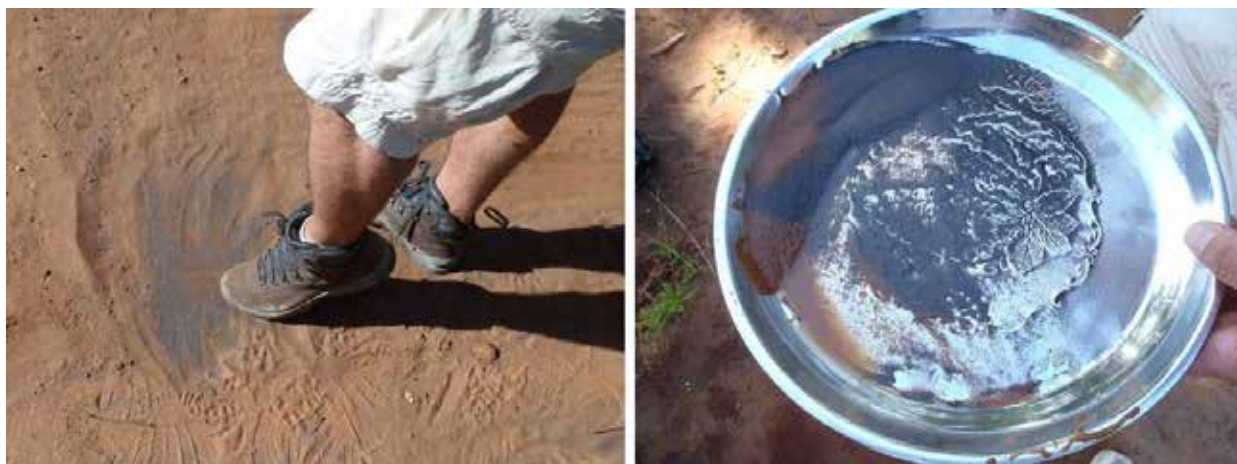
Figure 10 – Left: Exposure of high grade mineral sands at Tajiri and Right: Simple panning of the sand results in easy separation of the black heavy mineral content.
