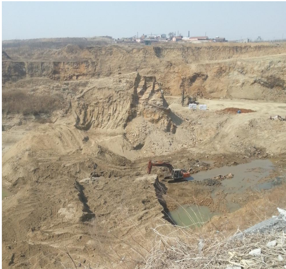
Figure 1 – The largest graphite mine in Shangdong Province, China. The rocks likely grade at 2-3% TGC and no visible graphite is obvious. Impurities in the deposit are a problem and need to be removed with acids. The mine is now relatively deep >60m and water ingress is a major problem.
